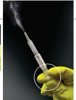
4. Compress bellows to generate smoke.
