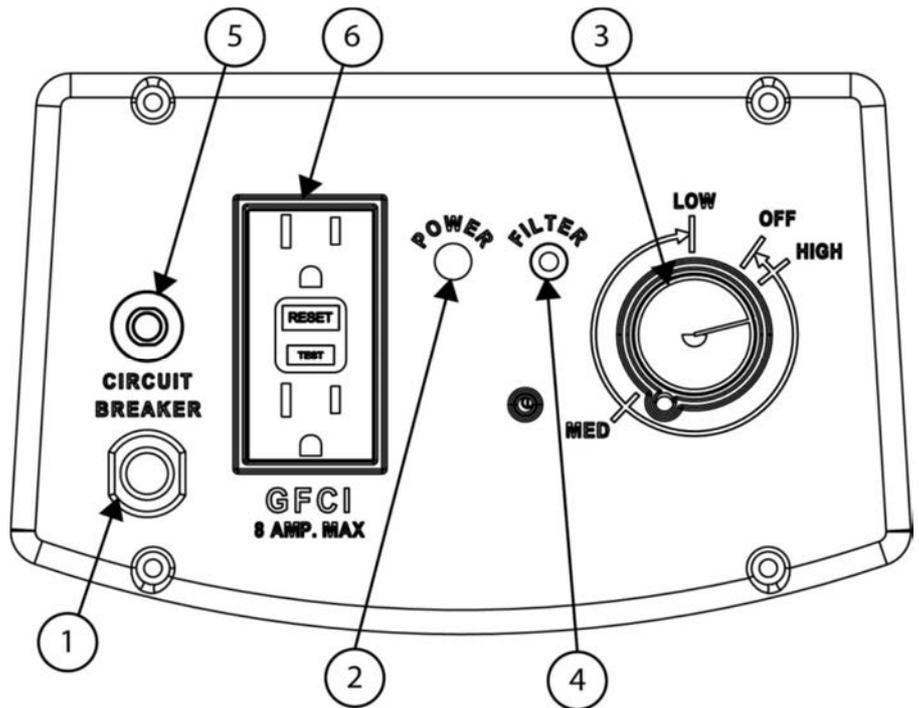
**Note:** If the equipment connected to the GFCI receptacle draws more than a total of 8 amps, the circuit breaker on the control panel and/or the building breaker will trip. This condition can be remedied only by reducing the total amperage draw.
