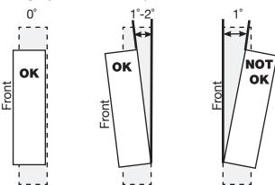
**Step 11.** Insert the dehumidifier into the center of the opening, allowing for a minimum of 1/8" clearance from framing on both sides. Additional insulation or sound dampening material (not provided) may be required if the dehumidifier cabinet contacts the studs, especially in applications involving metal studs.
