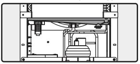
**Step 9.** Lift the unit and place it near the wall opening to route electrical wires and drain hose through appropriate knock outs.
