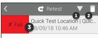
Touch **1** to reorder your failed results either ascending or descending. Touch **2** to delete results you don't plan on retesting. Touch a failed test result (as shown at **3** in the image) to see detailed information and perform a retest.
