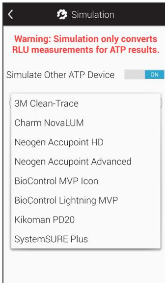
Turning on Simulation Mode converts the RLU results from ATP testing on your EnSURE Touch so that they simulate the results you'd get if you were using another system.
