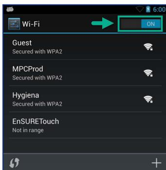
Turn on Wi-Fi if it is off. Select the wireless network to connect to. If you cannot find the wireless network to connect to in the list touch the Add (+) icon to manually add it.
