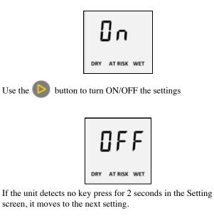
Pressing the **(U)** button, after you have entered the desired setting, will save the setting and move the screen to the next setting.
