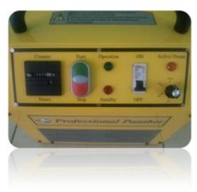
Time Counter (Hours); Remote Operation Key Switch Main switch with Over-Load Current protection; Start / Stop operation button; Power-ON (Green) light indicator; Ozone-generation ON (Orange) light indicator; Fault (Red) light indicator.
