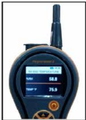
Figure 4: Hygromaster2 as a Hygrometer
