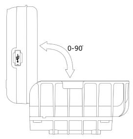
The display unit can be angularly adjusted from  $0^\circ$  to  $90^\circ$  for better viewing experience during measurement.
