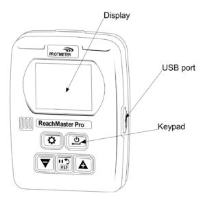
The display unit has a 2" screen to display the measurements from the sensor unit.
