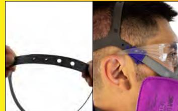
Make the head cradle bigger by moving pin locks to a wider position. This should drop blue buckle lower to fall under eyewear bar.
