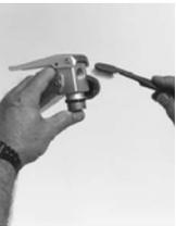
10. Clean outlet orifice with a small brush.
