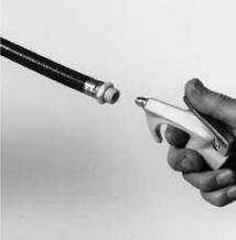
22. Check nozzle and/or hose for blockage and return to unit.
